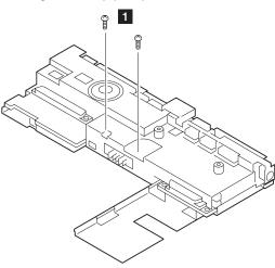
Turn the system board upside down. Then remove any metal tape holding the card.
